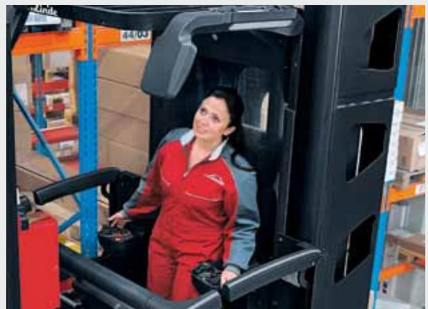
**Mirror module:** Best visibility onto guide rollers and over truck rear
