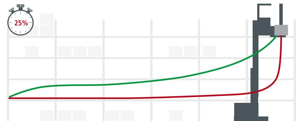
Optimised operation with storage navigation provides a time saving of up to 25%. The green line shows the shortest time using the fastest route and with as little energy used as possible.
