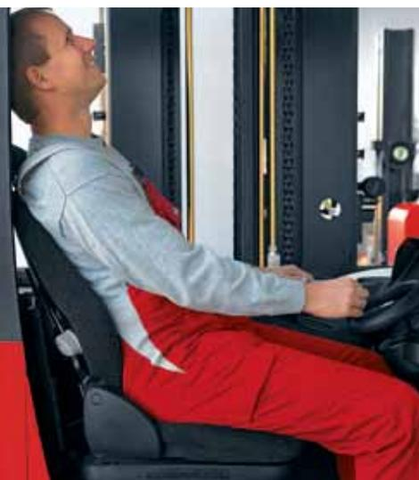
**Seat:** Hydraulically damped seat with lumbar support. Flexible and adjustable for visibility when placing or retrieving pallets. Available with a heater option.
