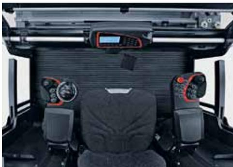
**The control units** can be quickly adjusted from standing to seated operation. Two-handed use is always assured via contact sensors
