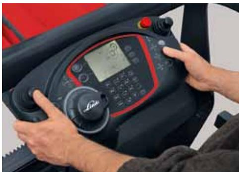
**The front Control Panel** can be easily adjusted for height, distance and tilt to suit each operator. The display shows all relevant truck operating data
