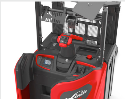
Ergonomic, height-adjustable tiller
