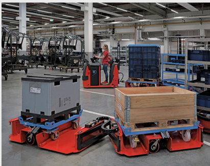
Minimal turning radius with six frames thanks to scissor drawbar
