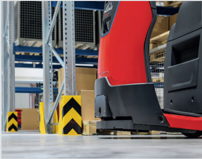
Linde BlueSpot™ and bumper including safety scanner
