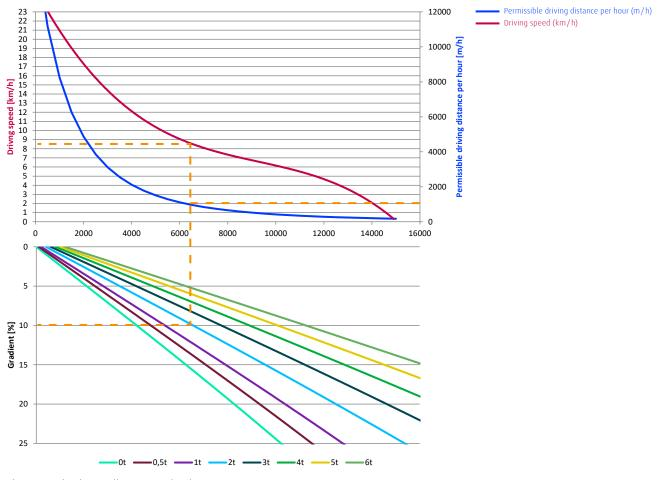
The example shown illustrates a load transporter transporting 2 t operating on a ramp of 10 %, maximum travelling speed reachable 8.5 km/h for a maximum travel distance per hour of 1.6 km (1600 m<sup>\*</sup>)
