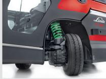
Coil spring and maintenance free braking system
