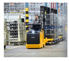
**Flexible on the train.** The Linde Load Trains consist of Linde P50 tow tractors and trolleys with all-wheel steering and wide lifting lips.
