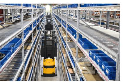
According to demand In the newly installed high-rack warehouse with 13 racking rows, the components required for the printing presses on the production line are picked on an order-by-order basis
