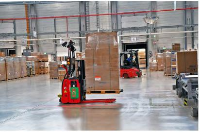
**Clear paths, maximum safety** Since the autonomous Linde units operate in a high-traffic area, they project red warning lines on the floor on either side of the truck, among other safety features.
