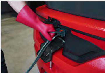
Disconnecting the charging plug
