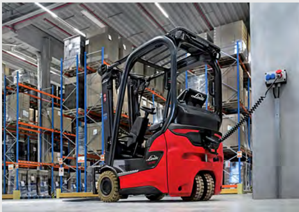
Charging cable of an integrated charger
